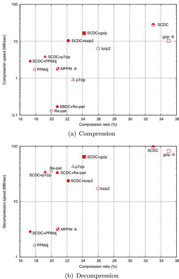
**FIGURE 5.** Space vs compression/decompression time trade-offs on corpus ALL. The x axis shows compression ratio (leftwards is better). The y axis (in logarithmic scale) shows compression and decompression speed (MB/sec), respectively (upper is better).
