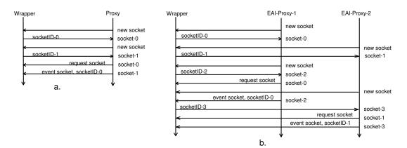
Figure 5: Sequence diagram of the connection protocol
