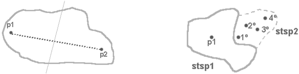
Fig. 6. On the left, we select p_1 and p_2 , and then divide the set. On the right, the merge step takes the objects according to their distances towards p_1 .
