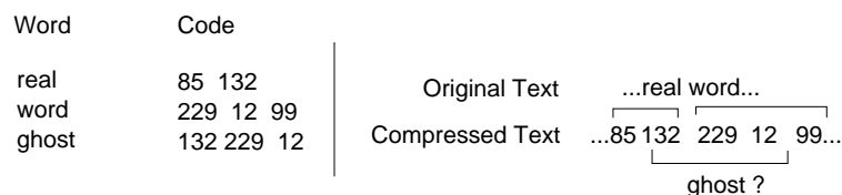
Fig. 3. An example where the codeword of a word is present in the compressed text but the word is not present in the original text. Codewords are shown in decimal notation.
