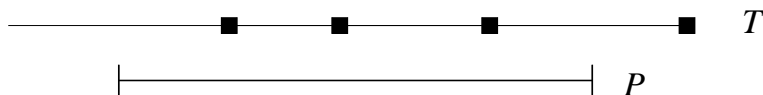
Figure 4: A window approach over LZ78/LZW compressed text. Black boxes are the explicit characters at the end of each block, while the lines are the implicit text that is represented by a reference.
