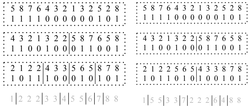
Figure 3: Wavelet tree/matrix representations of sequence S = 5876432132528 . On the left a levelwise WT, and on the right a WM.
