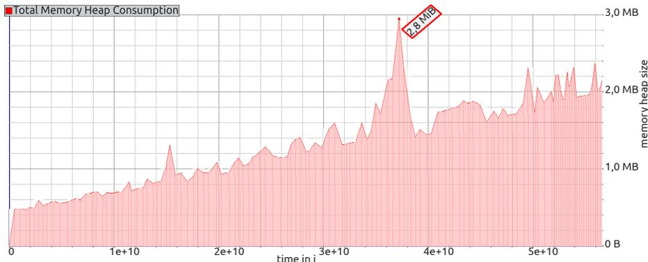
Figure 11: `valgrind` heap allocation profile for dataset `uk-2007-05`. The label `time in i` in the  $x$  axis denotes the number of instructions executed.
