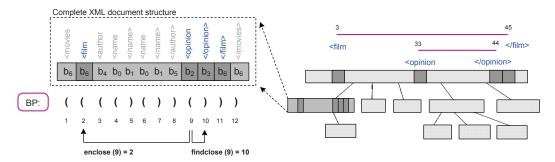
$\label{eq:Fig.3.Correspondence} Fig. 3. Correspondence between the root of the XWT subtree storing the document structure and a balanced parentheses representation.$
