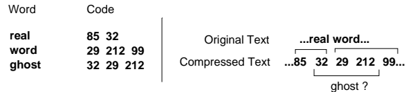
Figure 6: An example where the code of a word is present in the compressed text but the word is not present in the original text
