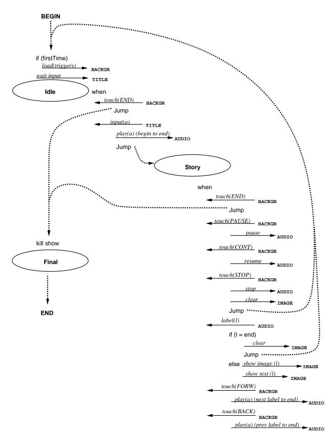
Figure 3: Automaton design for the interface.
