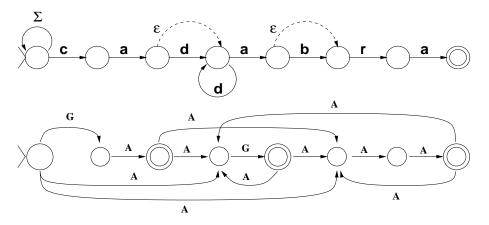
Figure 4: On top, an NFA to recognize an extended pattern with optional and repeatable characters. On the bottom, the NFA of a general regular expression.
