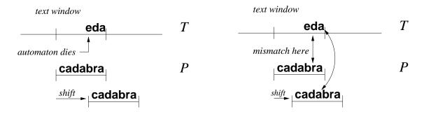
Figure 3: On the left, the BDM search process in a window. On the right, the same window processed by Horspool.
