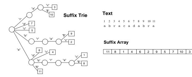
Figure 6: The suffix trie and suffix array for the text "abracadabra".
