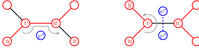
Figure 2: Left: If we process an edge (v, w) in T , then we move to w in our traversal of T and the next edge, (w, x) in this case, is also incident to the vertex v^* we are visiting in our traversal of T^* . Right: If (v, w) is not in T , then in T^* we move from v^* to the vertex w^* corresponding to the face on the opposite side of (v, w) in G . The next edge, (v, y) in this case, is also incident to w^* .
