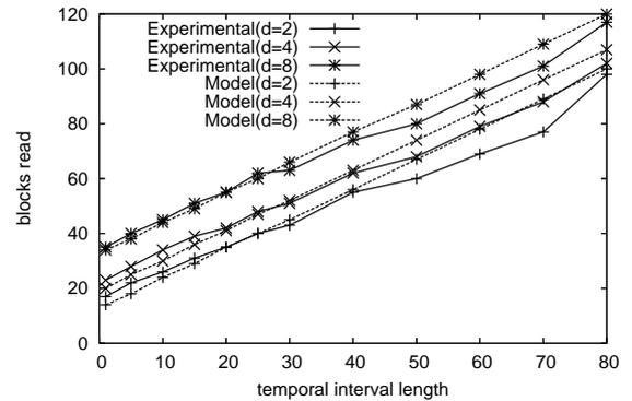
Figure 13: Estimation of the time cost of queries (10% change frequency and 6% in each dimension for query window)
